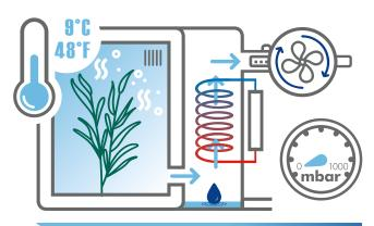
The water vapor is condensed by passing a "cold wall". The dried air goes out through the vacuum pump.
