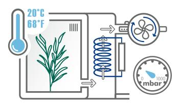
The vacuum pump starts and reduces the air pressure in the room from 1000 mbar to the desired pressure.
