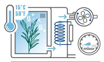
A small amount of water within the product will start boiling when pressure reaches temperature level of the product. This boiling process requires heat that is extracted from the product, enabling the cooling.
